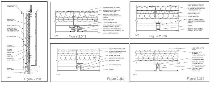
Mounting typically falls into either exposed or concealed fastener types. Whichever fastener type, ensure that the
