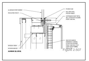
**PER curtain wall:** Bridge the AB/WRB line across to the back of the glazing pocket and maintain the thermal control layer. Connect the cladding to the curtain wall mullion covers. (figure 2.507)
