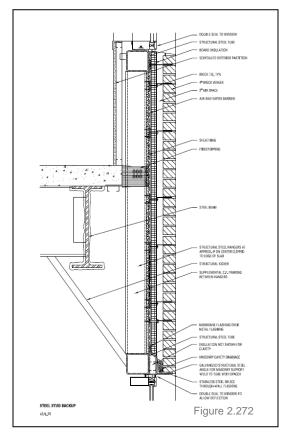
accommodate the more widely spaced and larger point loads. Note that every penetration of the AB/WRB should be detailed so that it can be properly sealed and inspected before installing the insulation. Be wary of anchors that supposedly seal through rigid insulation, the seal is frequently a gasket at the cavity face of the insulation, not at the proper location at the surface of the AB/WRB.
